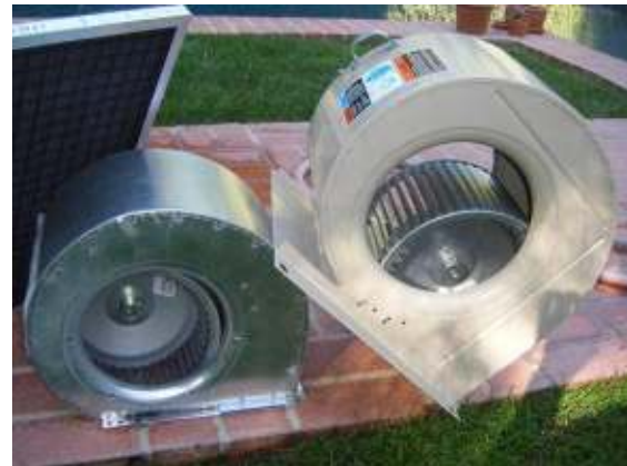
Motors will be disconnected and removed from direct-drive fans, and fans themselves will be taken out and washed with a mild, paint-safe detergent and water, then reinstalled as found.
