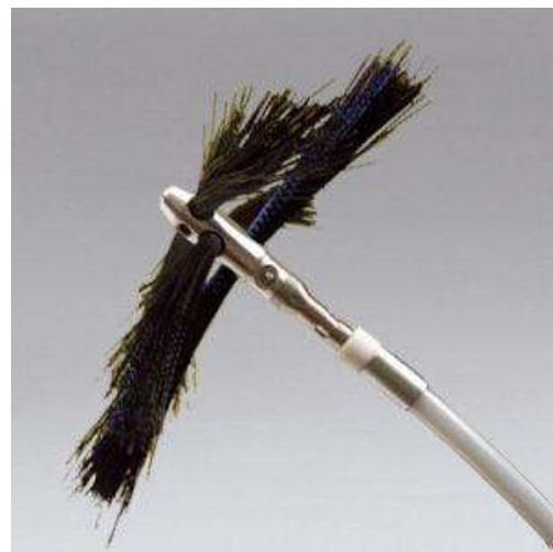
Duct augers, used to agitate contaminants, which are then removed by negative air.
